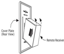
Position the receiver as shown in diagram to the left with lower tab on cover plate inserted into groove of receiver (Make sure ADJ hole and LEARN hole on cover plate properly aligns with remote receiver) Pull Receiver up and snap into top tab of cover plate.
