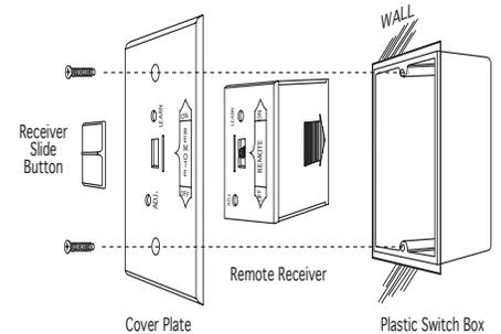
**NOTE:** The remote receiver will only respond to the transmitter when the 3-position slide button on the remote receiver is in the REMOTE position. If the system does not respond to the battery transmitter on initial use, see MATCHING SECURITY CODES, and recheck battery positions in the remote receiver.
