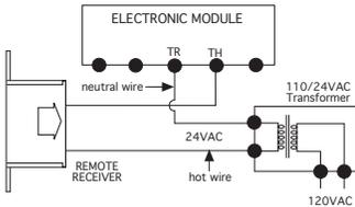
The remote control receiver can be connected, in series, to a 24VAC transformer to the TR (transformer) terminal on the ELECTRONIC MODULE. Connect the hot wire from the 24VAC transformer to either of the wire terminals on the remote receiver. Connect another wire (not included) between the other receiver wire terminal and the TH (thermostat) terminal on the ELECTRONIC MODULE.
