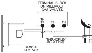
Operation of the remote receiver is similar to that of a thermostat in that both turn the gas valve on and off based on input signals. A thermostat's input signals are different temperatures. The remote receiver's input signals come from the transmitter.
