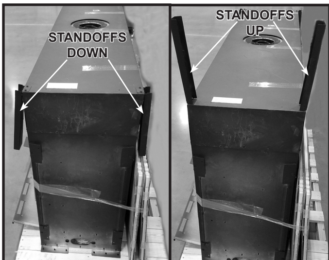
Standoff Shipping Position Standoff Installation Position
