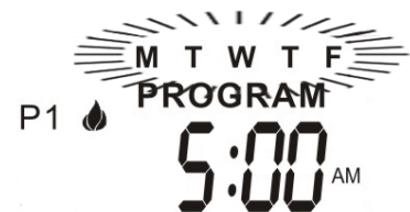
Fig. 23. Flashing weekday segments, time P1 and flame “ON” icon
