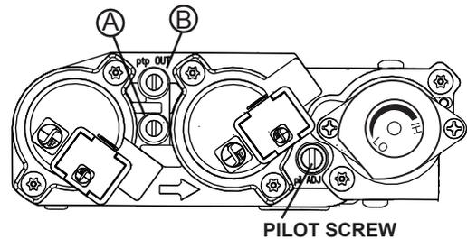
**After taking pressure readings, be sure to turn screws clockwise firmly to reseal. Do not overtorque.**
