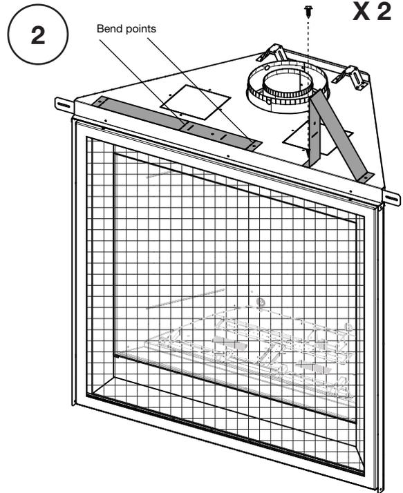
Use screws removed in step 1.
