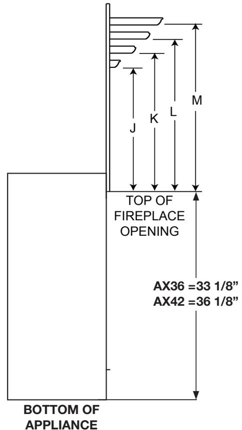
**ONLY if the Altitude™ X Heat Management System is installed, mantel clearances can be reduced.**
