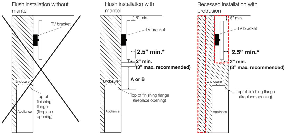
The volume of air must be added to the enclosure to accommodate the recessed area.
