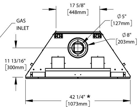
\* Finishing flange (the finishing flange defines the perimeter of the fireplace opening. Framing or finishing materials must NEVER encroach inside the finishing flange).
