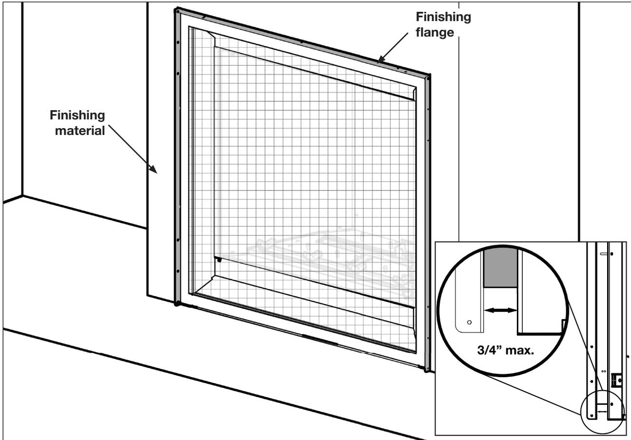
**Finishing flange** (the finishing flange defines the perimeter of the fireplace opening. Framing or finishing materials must **NEVER** encroach inside the finishing flange).
