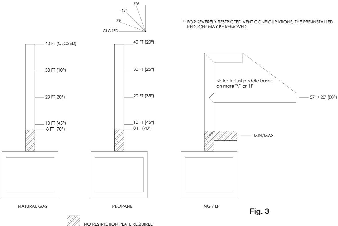
\*\* FOR SEVERELY RESTRICTED VENT CONFIGURATIONS, THE PRE-INSTALLED REDUCER MAY BE REMOVED.
