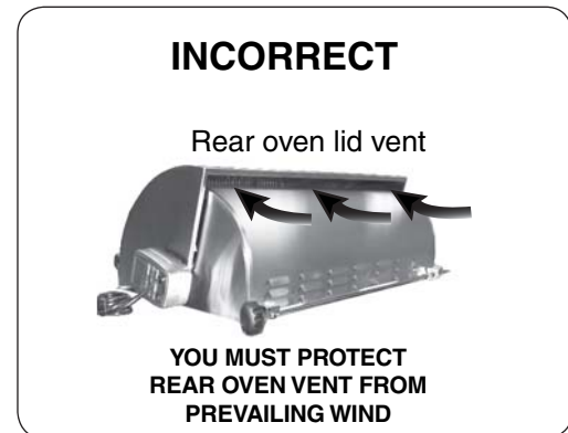
Fig. 12-2 Airflow direction - INCORRECT
