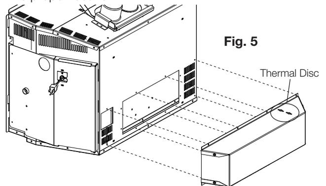
6. Loosen the thermal disc bracket (2 screws). Slide the bracket until the thermal disc is touching the rear of the firebox and then secure (**Fig. 6**).
