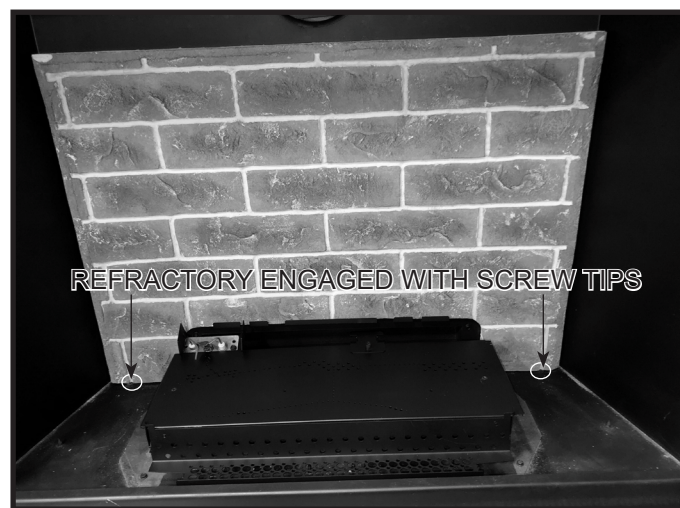
Figure 2 Install Rear Refractory
