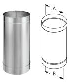
Use for a single-wall connector pipe. Requires 18" clearance to combustibles. Subtract 1  $\frac{1}{4}$ " from the length to calculate the installed length.
