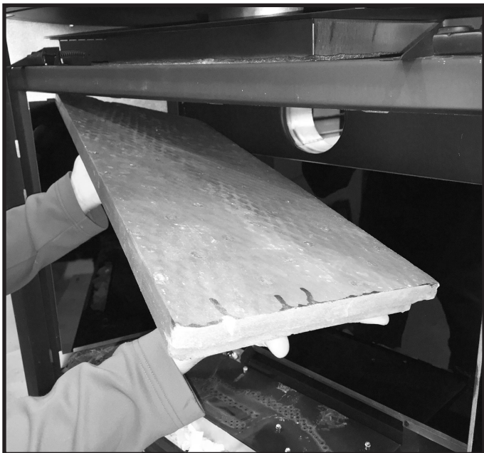
Figure 11 Install Top Refractory Panel
