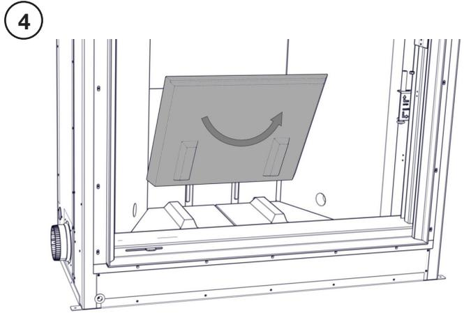
Place and slide the bottom rear firebrick against the wall.
