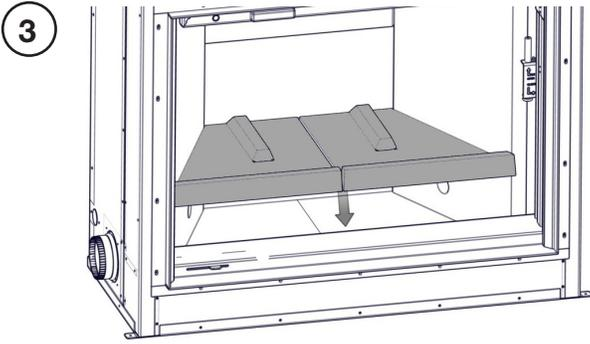
Install the bottom firebricks to lock all firebricks in place.
