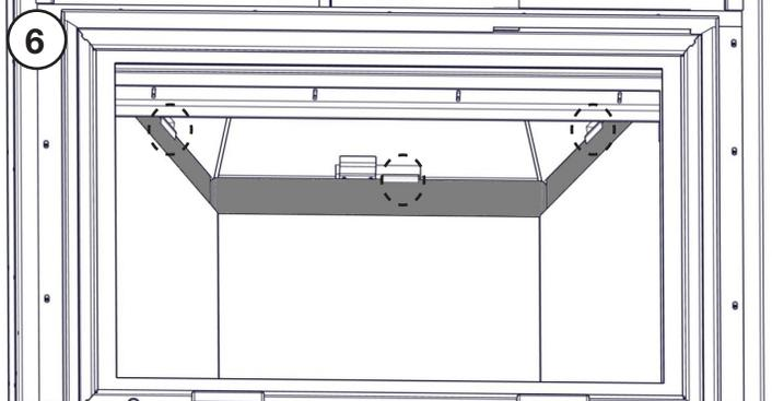
Install the 3 fiber panels and secure with retaining brackets.
