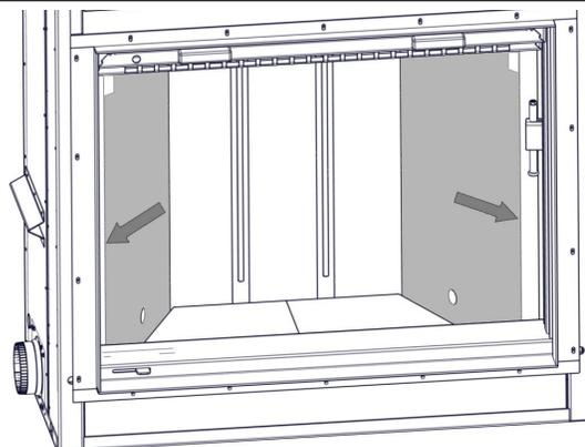
Tilt and install the right and left side firebricks against the wall. To install rear bricks, the side bricks must be pulled forward.
