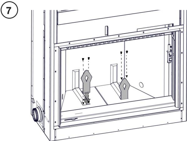
Install the andirons through the base bricks. Fasten with supplied hardware.
