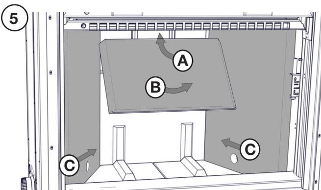
Place and slide the top rear firebrick against the wall (A and B). Push side bricks back to help hold rear bricks in place (C).
