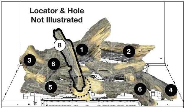
8. Place the locator on log #8 into the hole in log #1. Place the opposite end of log #8 on log #5.
