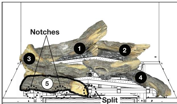
5. Place the 2 notches in log #5 on the 1st and 2nd grate posts, ensuring the notch on the split wraps around the grate at the 3rd post.
