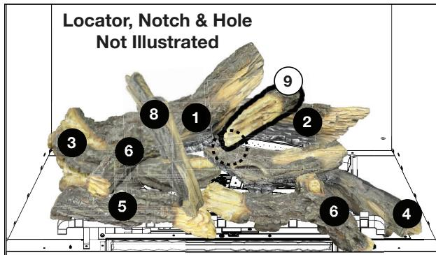
9. Place the locator on log #9 into the hole in log #4. Place the opposite end onto the notch in log #2.
