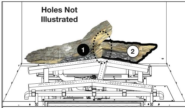
2. Place the holes in log #2 on B1 and B2, located on the rear log support. Ensure the left end of log #2 is behind log #1.
