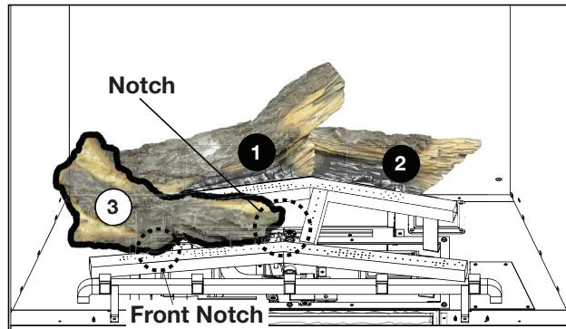
3. Place log #3 between the burners on the left side of the firebox. Engage the right notch with the pilot shield, and place the front notch on the front burner.
