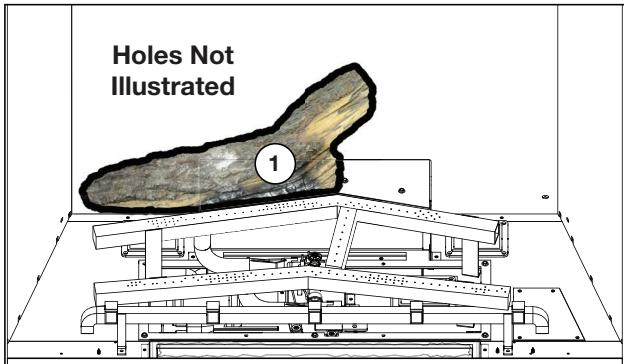
1. Place the holes in log #1 on A1 and A2, located on the rear log support.
