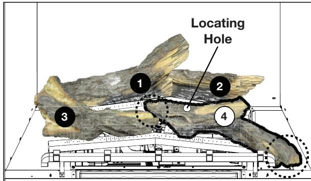
4. With locating hole facing up, place log #4 between the burners. Place the right end on the floor of the firebox and place the opposite end over the pilot. Shift the log slightly to the left to engage.
