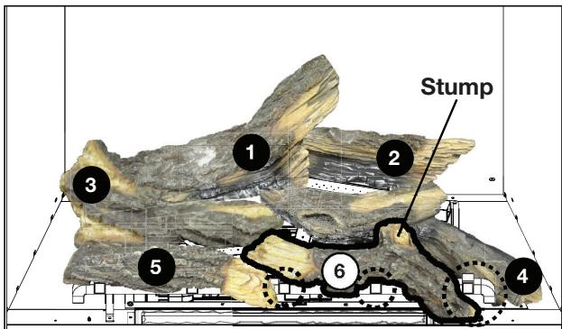
6. With the stump facing up, place the right end of log #6 on the floor of the firebox under the 5th grate post. Place the opposite end on top of the 3rd grate post.
