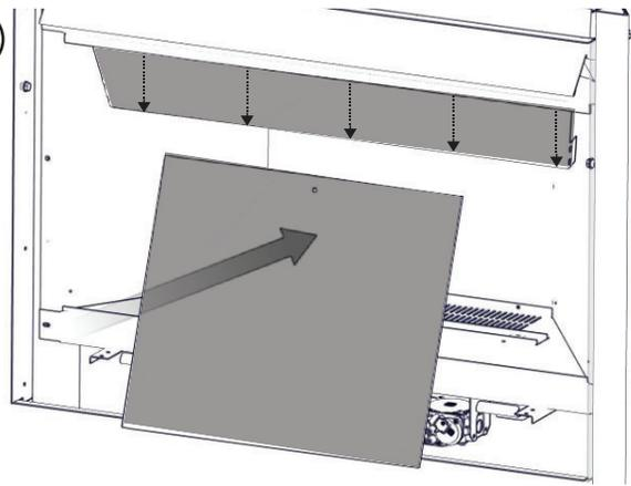
For ease of installation, remove the front baffle.
