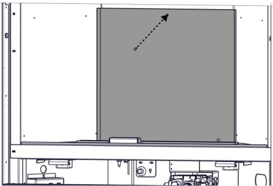
Secure the top of the rear panel using one screw (supplied).
