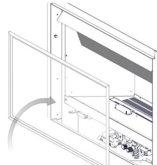
Reinstall media. Reinstall front baffle, if necessary. Reinstall door.
