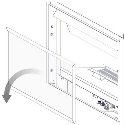
Place the door face down on a soft surface. Remove existing media.
