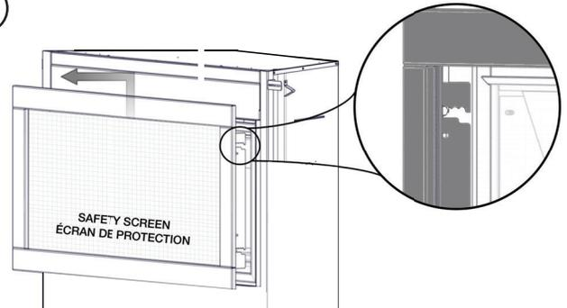
Disengage the four hooks to remove the safety screen.
