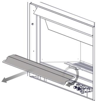
Lift the control cover up and remove from the appliance.
