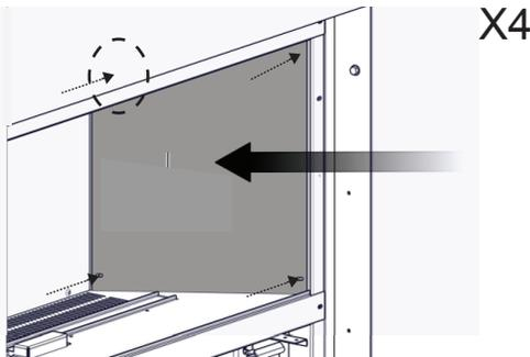
Secure the side panel using four screws (supplied).
