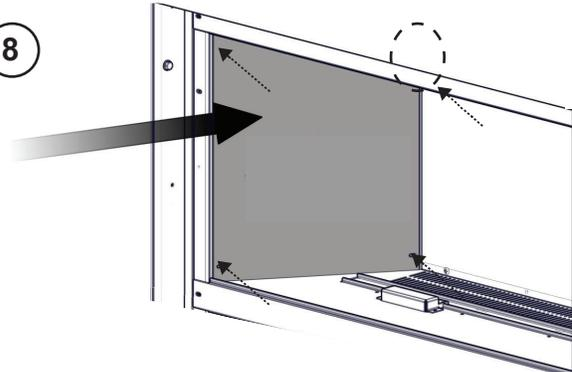
Secure the side panel using four screws (supplied).
