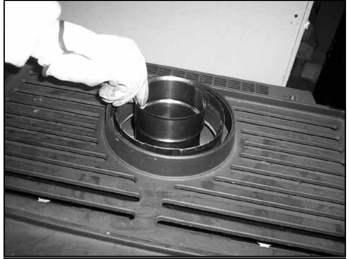
Figure 11 Install SLP-SAM Adapter
