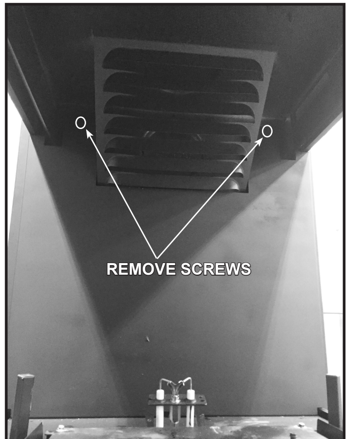
Figure 2. Remove Metal Refractory
