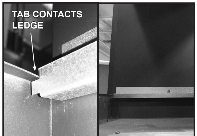
Figure 6. Install Refractory Channel - Side Opposite the Pilot
