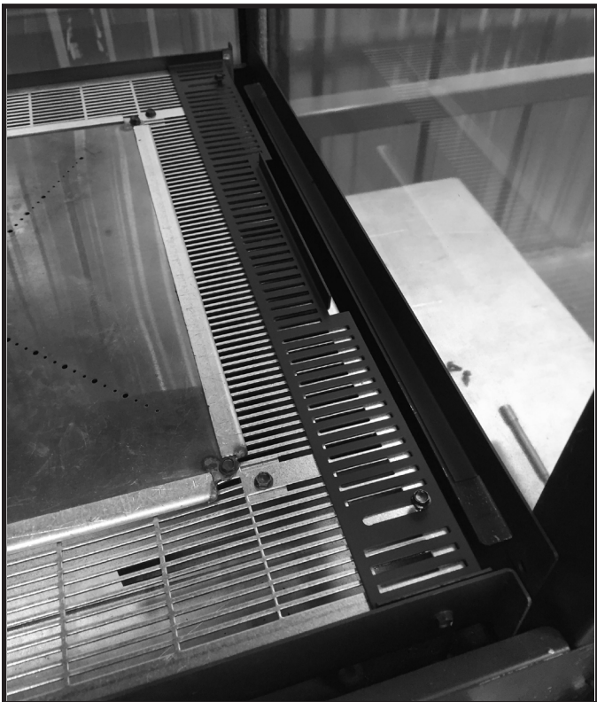
Figure 15. End Vanity Shroud in Place
