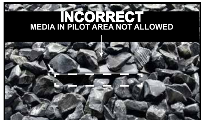
Figure 9.9 INCORRECT Media Placement
