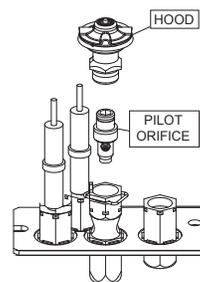
4. Loosen and remove the pilot tube fitting from the pilot housing. Replace the injector and re-assemble.
