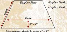
Measurements should be taken 6" – 8" inside firebox opening.
